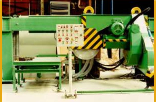
We offer you **manufacturing and delivery of Circular Saw M 800**. Strojírny a stavby Třinec developed **Numeric Controlled Circular Saw M 800 for cutting of refractory materials, stones and similar materials**. The diamond circular saw MGT-f 800 with easy replacement is applied for dry cutting of refractory materials as magnesite, chromiummagnesite, dolomite, corundum without water cooling.
