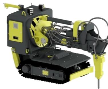
Strojírny a stavby Třinec a.s. for a long time work develop and product destroying and demolition manipulators for metallurgical plants. Manipulator is used for demolishing of wore refractory lining of ladles, torpedo cars, blast furnace runners, soaking pits and others. According to the purpose of usage, we are able to customize all technical parameters.
