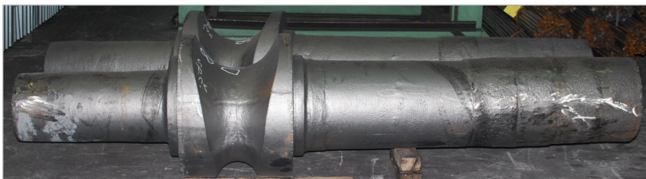
Casting of pilger roll with blanked groove
