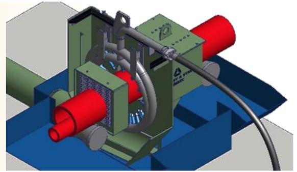
Strojírny a stavby Třinec, a.s. offer high pressure descaling, an effective method of scale removal from the surface of a hot metal semiproduct. This is the descaling of the metal product surface by high pressure water jet. It leads to improving the surface quality of the final product.
